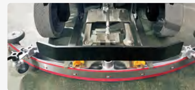
10 The wiper connecting rod structure is not easy to deform
